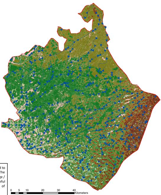
5 m Digital Elevation Model (DEM) has been used to generate surface topography of the district. The same product was used to extract natural drainage / gradients / flow directions. This map can be useful for determining route(s) for safe dewatering of flood water
